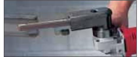
Grind and deburr ends of metal stock.
