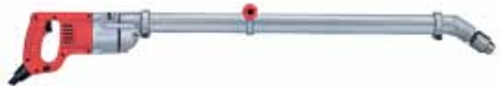
33° ANGLE DRIVE KIT 48-06-2860 For drill models 1001-1, 1007-1, 1101-1, 1107-6, 1109-24 and 1250-1. Stretches drilling reach up to 30 inches. Permits easy drilling of up to 2-9/16" dia. holes. Kit consists of an extension tube, side handle, drive shaft with hex sockets on both ends, two clamping collars and a 33° angle drive unit. Use 33° angle drive with the 30" extension only. 33° angle units operate at the same speed as the drill powering them.
